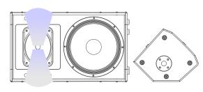
For Front of House configuration the narrow opening of the HF horn has to point downwards. For stage monitor configuration the HF horn has to be turned by 90 degrees, narrow opening pointing upwards. Remove the front grille and loosen the 4 screws of the HF horn. Turn the HF horn by 90 degrees and tighten the 4 screws. Then remount the front grille.
