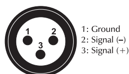
DMX-input XLR mounting-plug:
