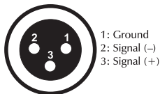
DMX-output XLR mounting-socket:
