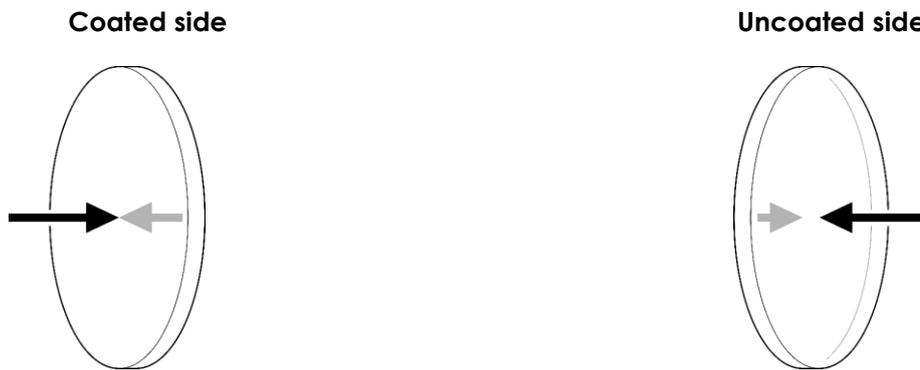
When an object is held up to the coated side, there is no space between the object and its reflection. The back edge of the gobo cannot be seen when looking through the coated side.
