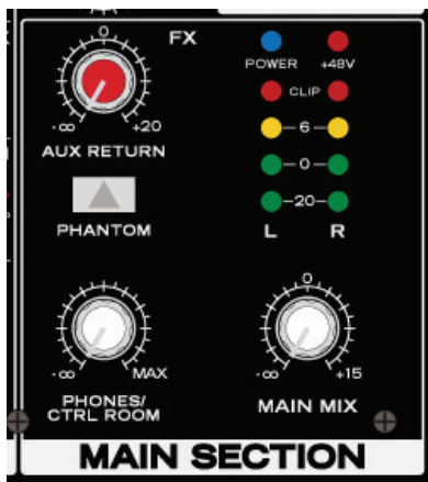
Fig. 2.4: Control elements of the main section
