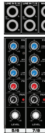
Fig. 2.2: Connectors and controls on the stereo channels
