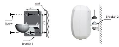
3. According to the installation plan in the adjustable range, adjust the most appropriate height, and then tighten the screws.
