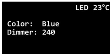
03) Turn the **manual dimmer control (13)** to adjust the intensity of the light. The adjustment range is between 0 and 255 (from 0 to 100 %). The current value of the dimmer is displayed on the screen.
