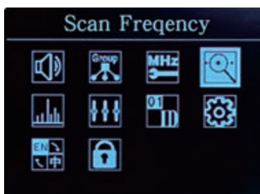
Scan Frequency: Auto scan to find and set a best frequency in a working environment
