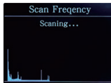
Scan Frequency: Auto scan to find and set a best frequency in a working environment
