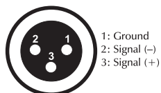
DMX-output XLR mounting-socket:
