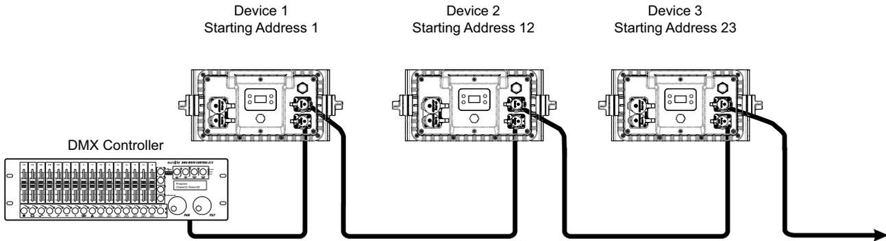
A DMX512 data link is required in order to control the device via DMX. The device provides special DMX connectors, which are designed according to protection class IP65. Matching DMX connection cables with special plugs are optionally available. When not in use, make absolutely sure to close the connections with the rubber sealing caps to prevent moisture and dirt from penetrating.
