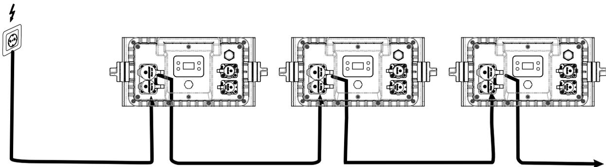
The device uses an auto-range power supply that accepts input voltages between 100 und 240 volts. The power connectors are designed according to protection class IP65. Matching connection cables with special plugs are optionally available. When not in use, make absolutely sure to close the connections with the rubber sealing caps to prevent moisture and dirt from penetrating.
